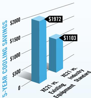
SEER stands for "Seasonal Energy Efficiency Ratio" and is a measure of a central air conditioner's efficiency and performance. The higher the SEER, the greater your energy savings. Typical SEER ratings range from 13 to 18, but the XC21 carries ratings as high as 21.20.
