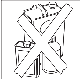
Fig. 4 - NO combustible materials near furnace
